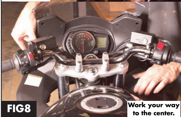
Fig 8. Now you are ready to separate the inner fairing from the bike. Start from the two tail ends and start dislodging and working your way to the inside.
