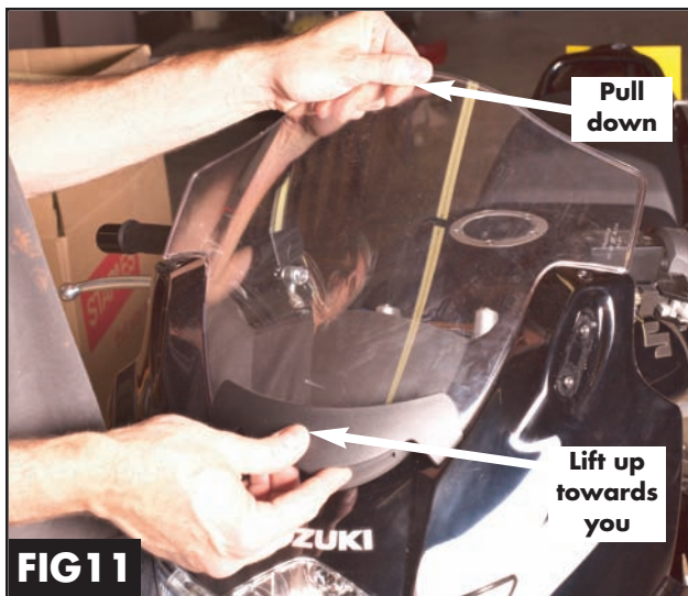
Fig 11. Prepare to remove windscreen. Hold the windscreen top and bottom as shown. First lift bottom of windscreen up towards you. While pulling top of screen towards the bike tank. See FIG11. Be careful not to exert too much force!
