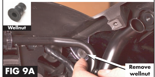
Fig 9A. After removing both allen fastener, remove the wellnut for easier screen removal. (For Both Sides) See FIG9A.
