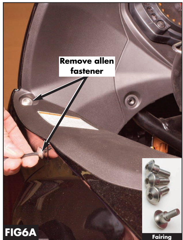
Fig 6A. On the same plastic fairing, there are 4 silver allen fastener located on the top and the sides. (For Both Sides) Note: The finish allen screws are in Silver.
